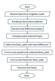
Figure 3.Reactive routing protocol for proposed system
