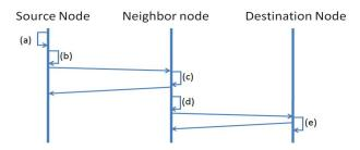
Figure 4. Proactive Routing Protocol in WMN (Sequence diagram)
